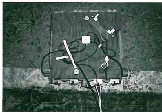
Fig. 2. Plywood boxes with elements were used to heat the hull of Seafresh 1 and kill Undaria gametophytes (photo: New Zealand Diving and Salvage Ltd.).
