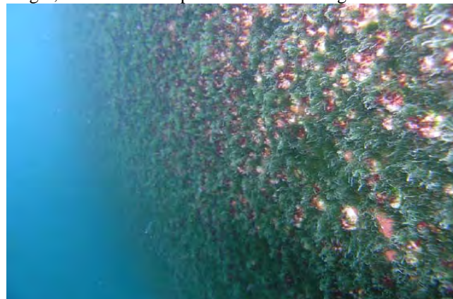
Figure 4 – Fouling Equivalent to 80% coverage of barnacles interspersed with weed
