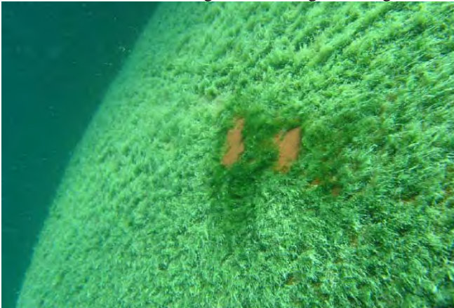
Figure 6 – Weed Fouling as can be found on upper faces of sonar domes
