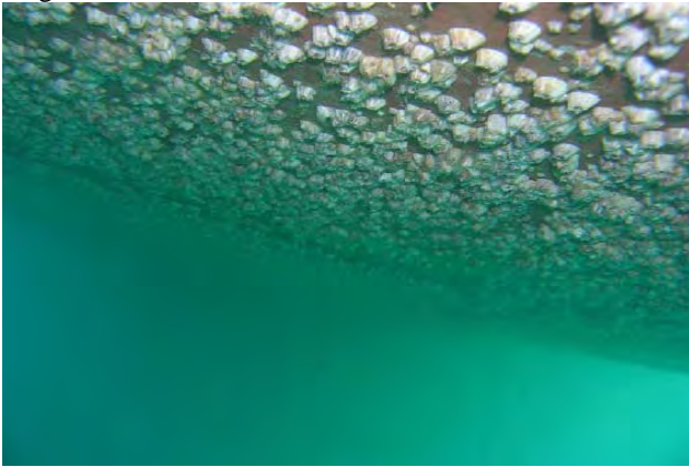
Figure 5 – Barnacle Fouling of 70-80%, note little weed present due to reduced light under the hull
