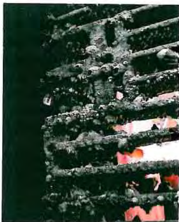
Seachest Grate: Barnacle fouling -seawater intake grate.
